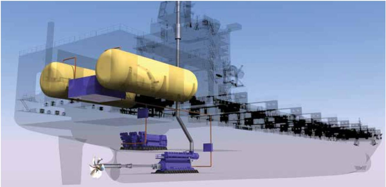
With ship operators facing economic pressures from fuel costs, combined with impending regulations aimed at reducing exhaust gas emissions, particularly for sulfur oxide (SO<sub>x</sub>) LNG-fueled marine propulsion systems are finding favor.
